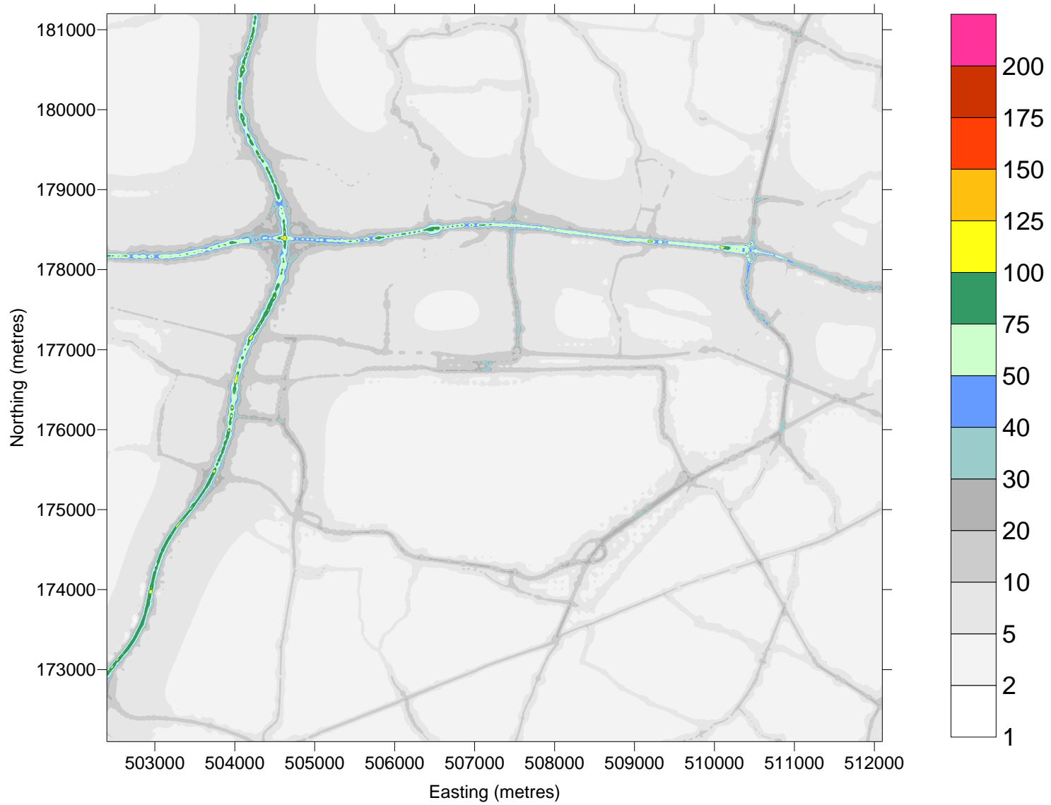
Figure 10.29 2030MM predicted NO_x concentration in \mu g/m^3 around Heathrow due to road sources
